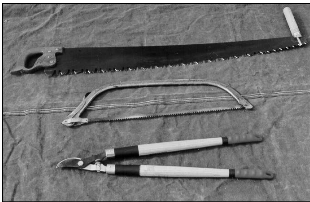
Top: one- or two-person crosscut saw Middle: bow saw Bottom: nippers or pruning shears
